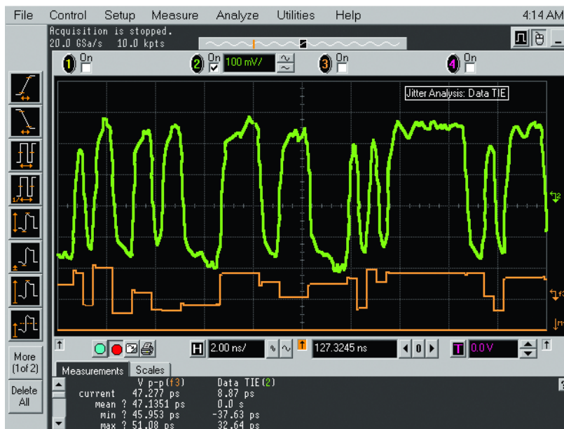
Figure 12. ISI due to reflections
