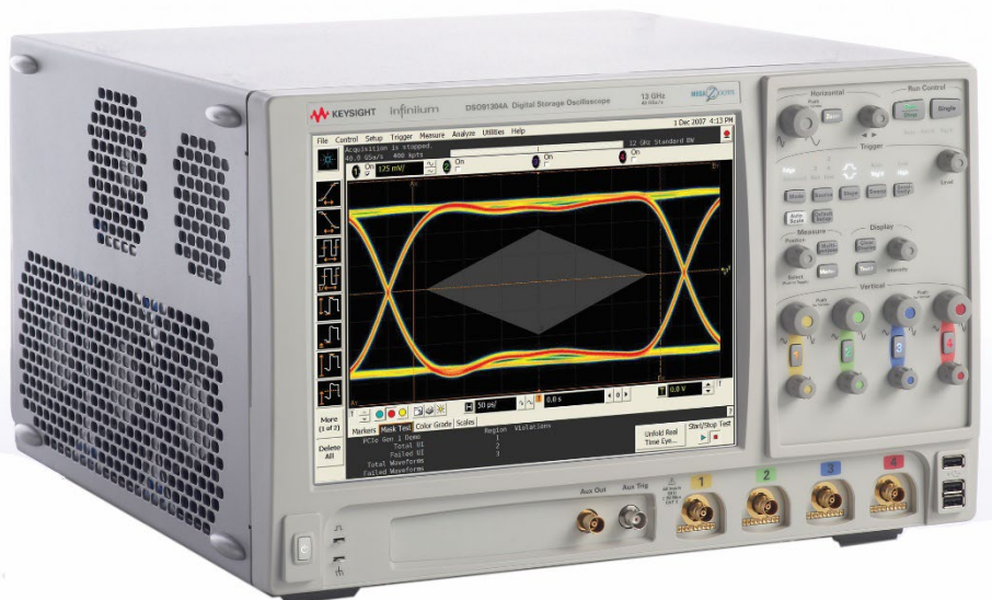
Figure 19. Keysight's 90000 12 GHz real-time oscilloscope
